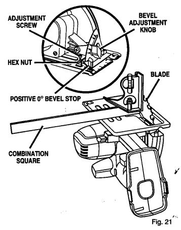
Your saw has a positive 0° bevel stop, that has been factory adjusted to assure 0° angle of your saw blade when making 90° cuts. However, misalignment can occur during shipping.
